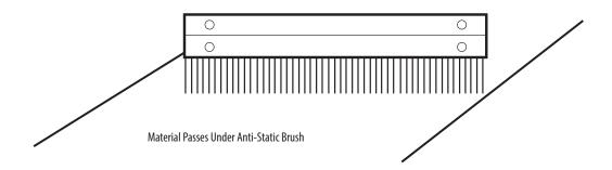
The TAKK Anti-Static Brush must be grounded. A good ground can be achieved by mounting the bar directly to a metal part of a grounded machine frame or by running a separate copper ground wire to either end of the Anti-Static Brush and an established electrical ground, such as an electrical box, conduit, etc.
